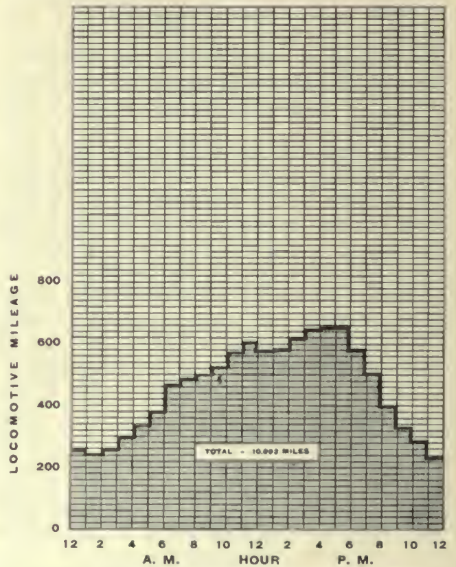
FIG. 405. TRAFFIC DIAGRAM. Locomotive-Mileage for the Average Day for Steam Operation in Freight Transfer Service within Area of Investigation.
